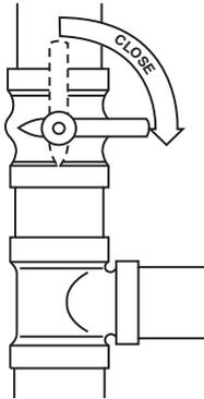
**Fig. 17 - Close the External Manual Valve**
