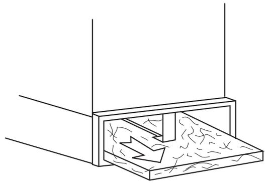
**Fig. 24 - Removal of Filter from Bottom Blower Cabinet**
